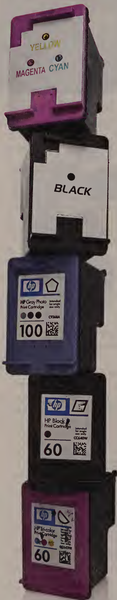
STICKERS IN THE InkTec kit (top two cartridges) help you find the holes for injecting ink.
